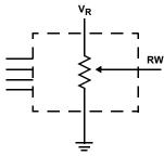
Three terminal Potentiometer; Variable voltage divider
