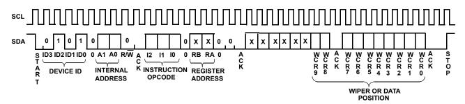
FIGURE 4. FOUR-BYTE INSTRUCTION SEQUENCE (WRITE OR READ FOR WCR OR DATA REGISTERS)
