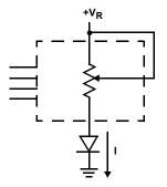
Two terminal Variable Resistor; Variable current
