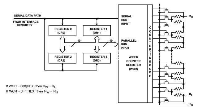
FIGURE 1. DETAILED POTENTIOMETER BLOCK DIAGRAM
